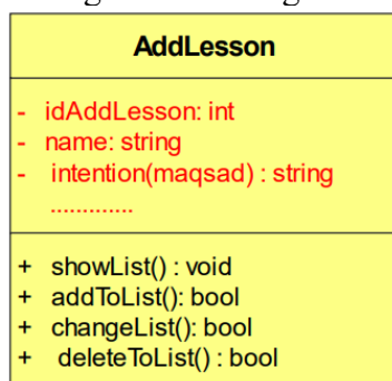
2-rasm. “AddLesson” sinfining xossalari va metodlarining diagrammasi
